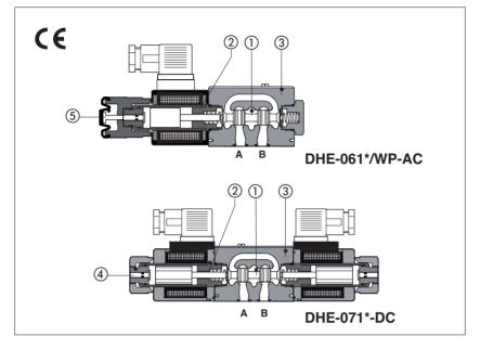
Spool type, two or three position direct operated valves with high performance threaded solenoids certified according the North American standard cURus.
