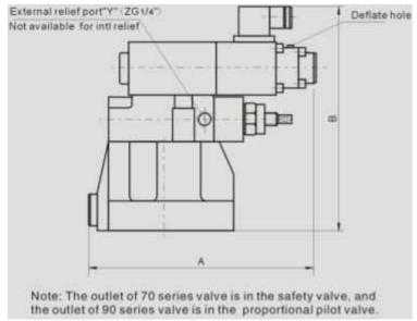
Note: The outlet of 70 series valve is in the safety valve, and the outlet of 90 series valve is in the proportional pilot valve.
