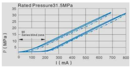
BY03, 06, 10, The result is tested under 271/min
