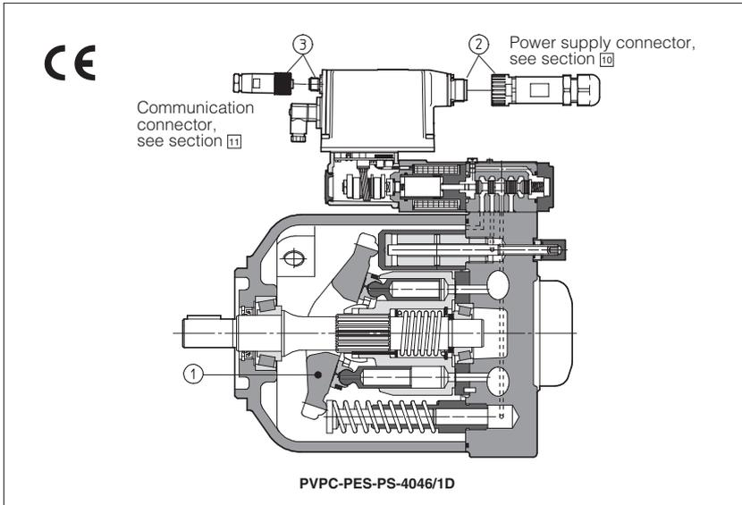
These digital drivers are integral to the Atos variable displacement axial piston pumps type PVPC. They control in closed loop the pump swashplate position ① and the system pressure according to the electronic reference signals realizing a P/Q regulation.
