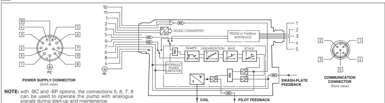
**NOTE:** with -BC and -BP options, the connections 5, 6, 7, 8 can be used to operate the pump with analogue signals during start-up and maintenance.
