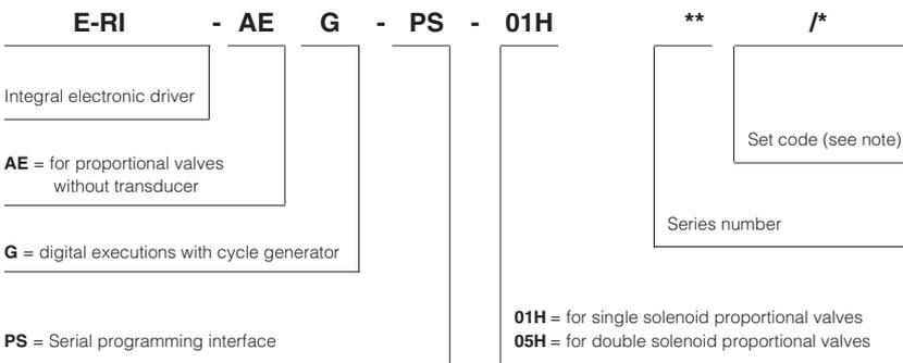
**Note:** the set code identifies the correspondance between the digital integral driver and the relevant valve; it is assigned by Atos when the driver is ordered as spare part.
