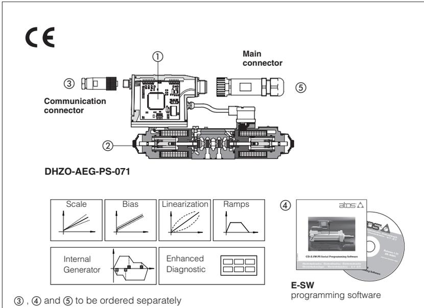
E-RI-AEG integral digital drivers ① supply and control the current to the solenoid of Atos proportional valves without transducer, according to the electronic reference input generated internally by means of six on-off input signals.
