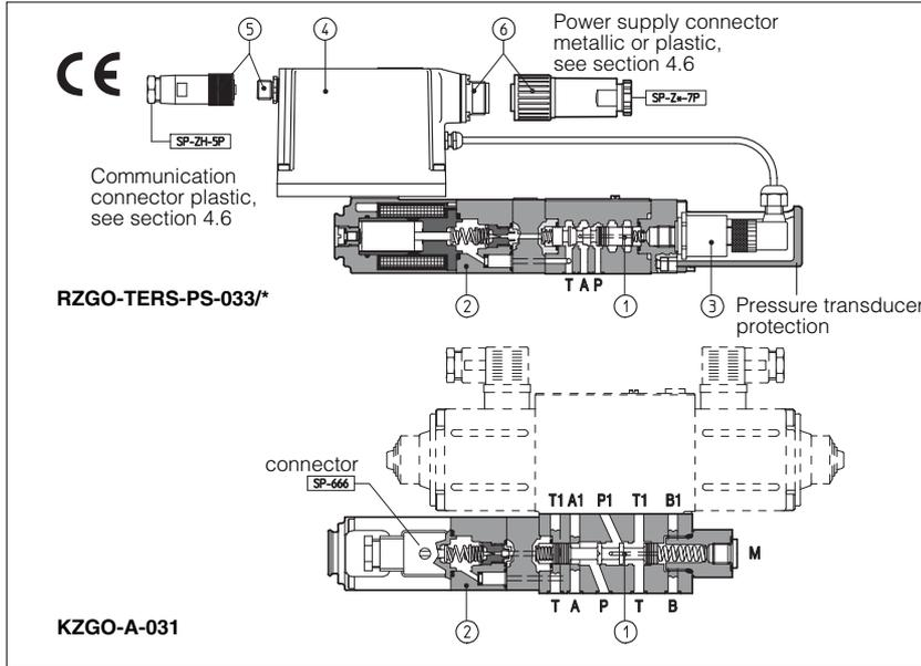
They are proportional pressure reducing valves, 3-way, pilot operated, available in two different executions:
