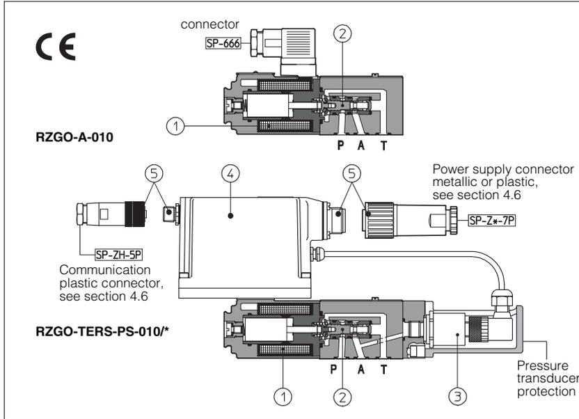
RZGO are 3-way proportional pressure reducing valves, direct operated with pressure regulation proportional to electronic reference signal.
