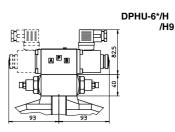
Mass of valve with option /H\*: kg 42,4 (one solenoid) kg 43,1 (two solenoids)
