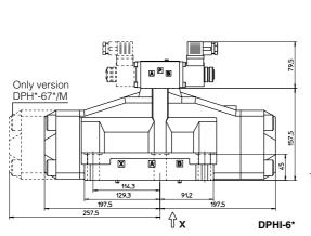
Mass of basic versions: kg 42 (one solenoid) kg 42,3 (two solenoids)
