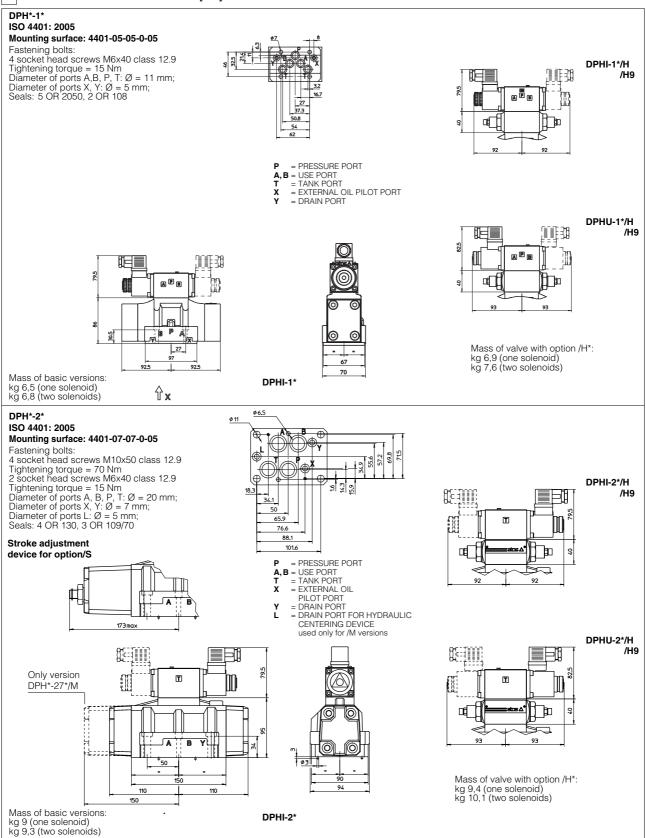
Overall dimensions refer to valves with connectors type SP-666
