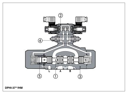
DPHI and DPHU are spool ① type, two or three position directional two stage solenoid valves designed to operate in oil hydraulic systems.
