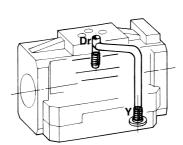
Internal piloting: blinded plug SP-X500F in X;
