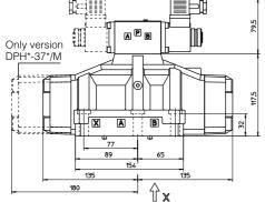
Mass of basic versions: kg 14 (one solenoid) kg 14,3 (two solenoids)
