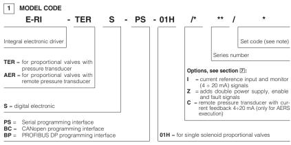
**Note:** the set code identifies the corrispondance between the digital integral driver and the relevant valve; it is assigned by Atos when the driver is ordered as spare part.
