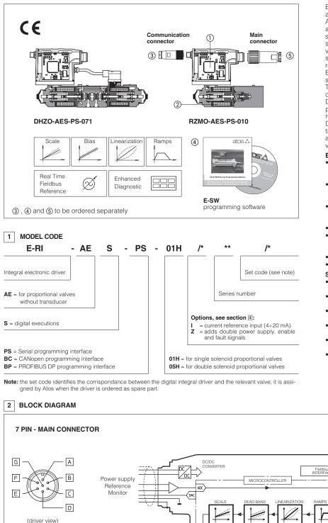
E-RI-AES integral digital drivers ① supply and control the current to the solenoid of Atos proportional valves without transducer, according to the electronic reference input signal. The solenoid ② proportionally transforms the current into a force, acting on the valve spool or poppet, against a reacting spring, thus providing the valve's hydraulic regulation.
