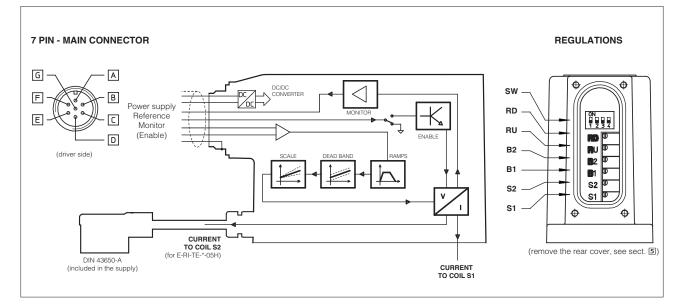
E-RI-AE integral analog drivers ① supply and control the current to the solenoid of Atos proportional valves without transducer, according to the electronic reference input signal.
