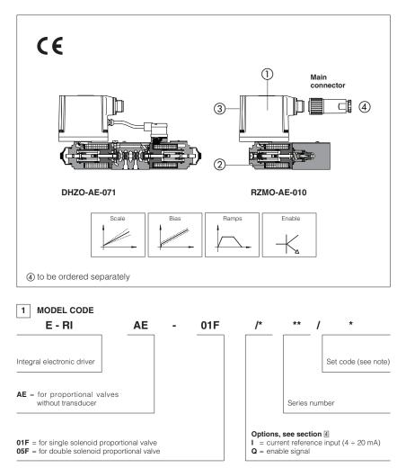
Note: the set code identifies the corrispondance between the integral driver and the relevant valve; it is assigned by Atos when the driver is ordered as spare part.
