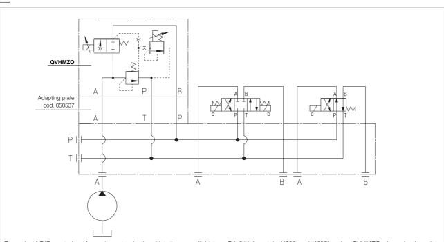
Example of P/Q control performed on standard multistations manifold type BA-214 (see tab. K290 and K295), using QVHMZO plus adapting plate cod. 050537
