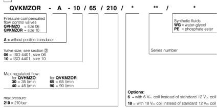
QVHMZO and QVKMZOR are proportional valves, direct operated, which provide indipendent pressure and 3-way compensated flow controls according to the electronic reference signals.
