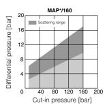
The graphs show, according to the set cut-in pressure, the pressure difference between the insert and the at-rest positions of the pressure switch electric contacts.
