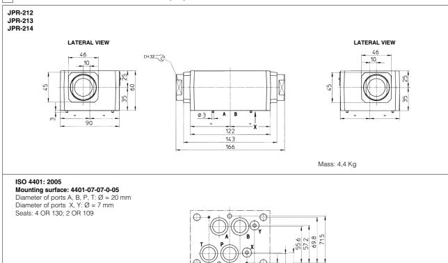
Fastening bolts: n° 4 socket head screws M10 and n° 2 M6. The lenght depends on number and type of modular elements associated.
