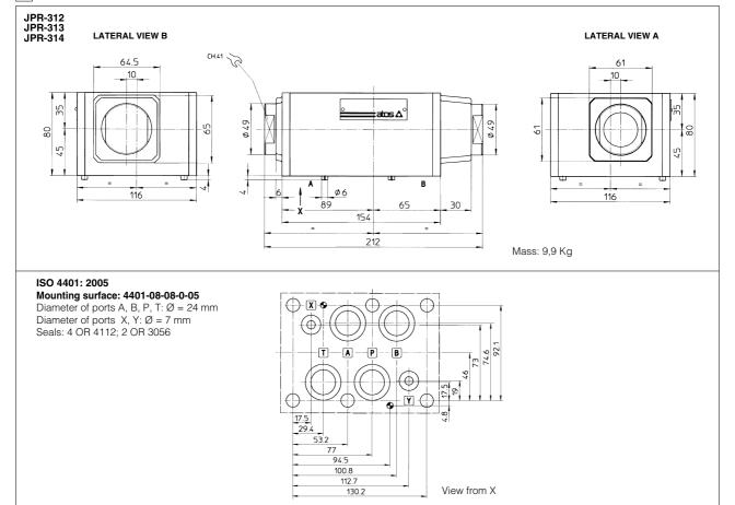
$Fastening\ bolts:\ n^{\circ}\ 6\ socket\ head\ screws\ M12.\ The\ length\ depends\ on\ number\ and\ type\ of\ modular\ elements\ associated.$
