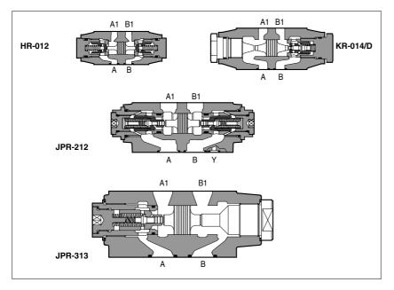
HR, KR are check valves available as direct or pilot operated models. JPR are pilot operated check valves.
