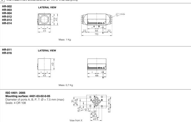
Fastening bolts: n° 4 socket head screws M5. The lenght depends on number and type of modular elements associated.
