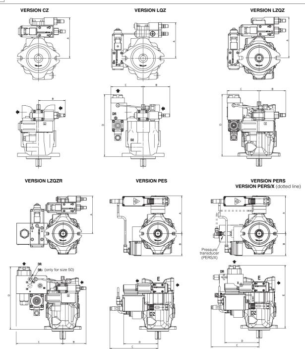
① = Regulation screw for max displacement. Adjustable range 50% to 100% of max displacement (not available for versions PES, PERS and PERS/X). In case of double pump the regulation screw is not always available, please contact our technical office.
