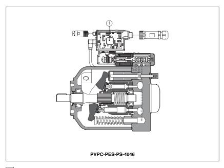
pumps type PVPC, can be supplied with advanced electrohydraulic proportional controls: · open loop pressure control;
