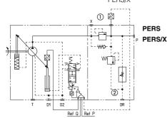
Digital P/Q controller integrates the combined pressure and flow regulation with the electronic max power limitation.
